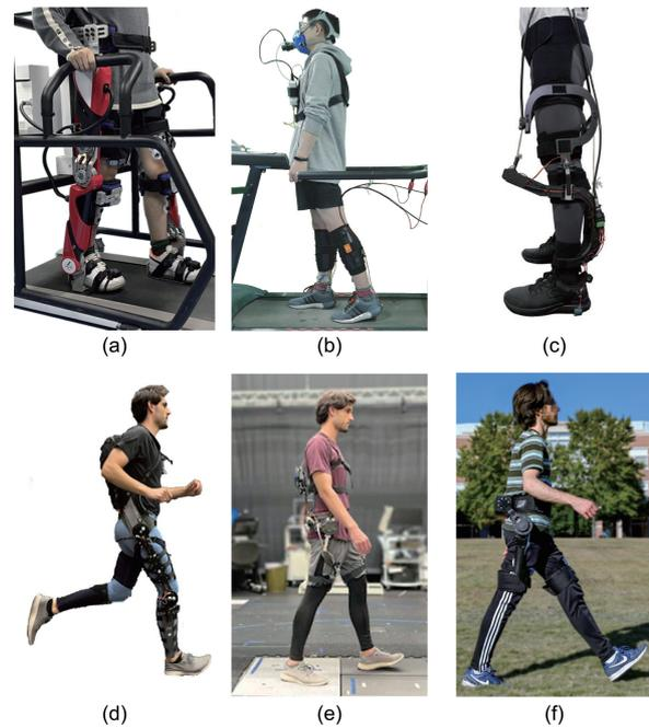
**Figure 13.** Innovative exploration of various exoskeleton designs and control strategies: (a) hip-knee-ankle exoskeleton with series elastic actuators; (b) soft exosuit; (c) ligaments-inspired knee exoskeleton; (d) task-agnostic exoskeleton control; (e) unified exoskeleton control; (f) sim2real framework for the exoskeleton.
