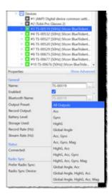
If Global Angle is selected, the capture rate is 225 Hz. If Global Angle is cleared, the capture rate is 1125 Hz. If HighG only is selected, the capture rate is 1600 Hz.
