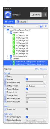
When Vicon IMUs are connected into Nexus, in the Properties pane in the Status section, their status is displayed as Connected and the sensor coordinate system is displayed in the bottom right of the 3D Perspective view (if the Global Angle axis is enabled – see Select the required axes, page 258).
