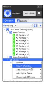
c. In the Whitelist Devices dialog box, select only the names of the IMU sensors that you want to connect (to find names from a long list, use the filter with standard wildcards, such as asterisk \* and question mark ?), then click Check Selected and click OK.
